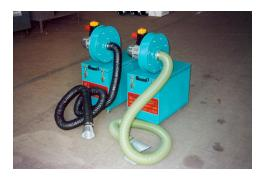
**SALDEPUR AP**: unit for suction, differentiated filtering and fume adsorption, with a capacity of 500 m3/h and motor kW 0.37 with 13 Kg of special type C3 active charcoal. The photo shows two units: one with a black anti-static flexible tube Ø 80 mm; the other with a green PVC flexible tube Ø 80 mm and a CCM type hood in galvanised sheet with a magnet to fasten metal surfaces.
